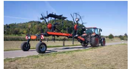
Transport height below 4.0m.
