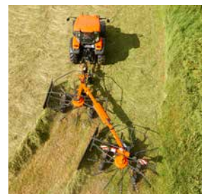
Both rakes are capable of placing small narrow swaths for hay crops.
