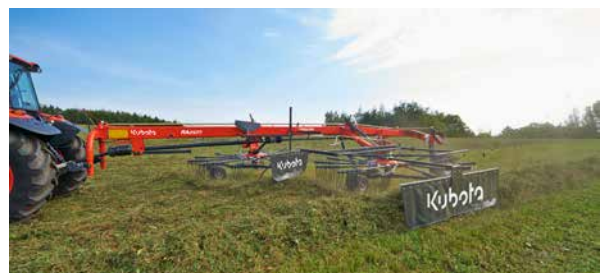
The low position of the rear frame ensures excellent stability.
