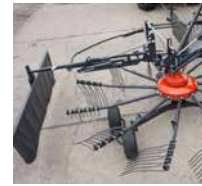
Automatic fold-able swath board with parking stand.
