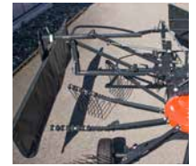
Automatic fold-able swath board with parking stand.
